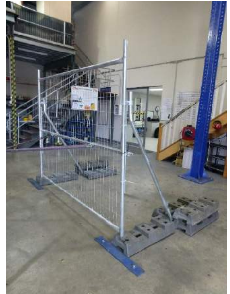
FIG. 5 SIMULATED WIND LOAD TEST SET UP ‘PERPENDICULAR’ BRACING
