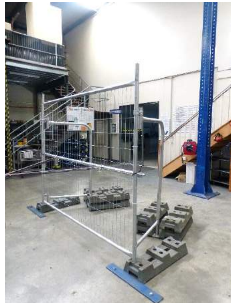
FIG. C8 WIND LOAD TEST SET UP ANGLED 'F-BRACE' BACK BRACE AND FENCE PANEL LOCATED AT THE EDGE FOOT BLOCK HOLES
