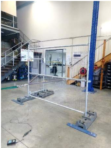
FIG. C3 WIND LOAD TEST SET UP PERPENDICULAR F-FRAME BACK BRACE AND FENCE PANEL LOCATED AT THE CENTRE FOOT BLOCK HOLES
