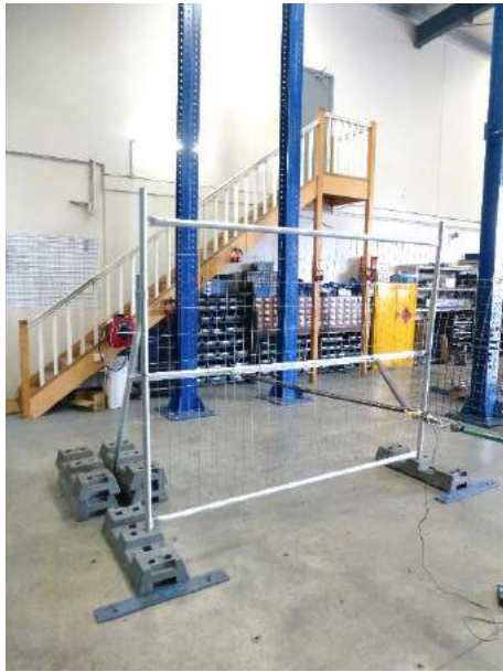
FIG. C5 WIND LOAD TEST SET UP PERPENDICULAR 'HEAVY DUTY' BACK BRACE AND FENCE PANEL LOCATED AT THE CENTRE FOOT BLOCK HOLES
