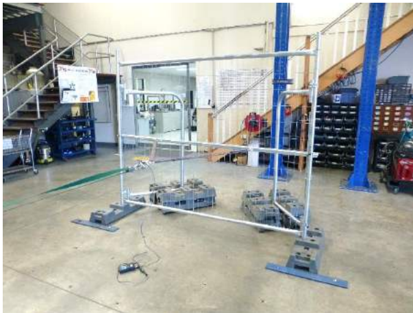
FIG. C7 WIND LOAD TEST SET UP ANGLED 'F-BRACE' BACK BRACE AND FENCE PANEL LOCATED AT THE CENTRE FOOT BLOCK HOLES
