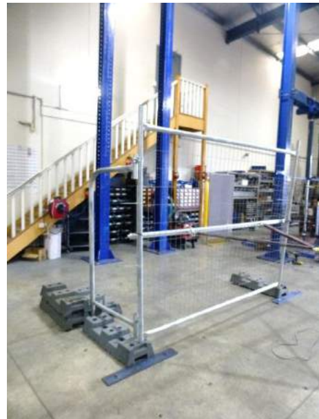
FIG. C4 WIND LOAD TEST SET UP PERPENDICULAR F-FRAME BACK BRACE AND FENCE PANEL LOCATED AT THE EDGE FOOT BLOCK HOLES
